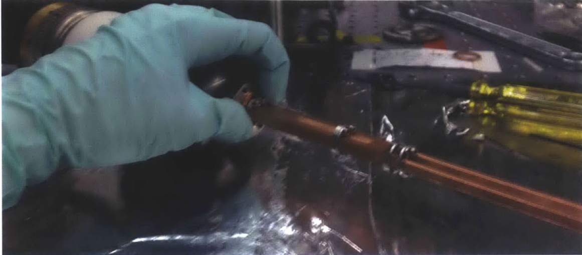
Figure 5-20: Installation and alignment of the TWT structure onto the anode. The alignment surface is held in place with 4 screws on the back-side of the copper anode piece.
