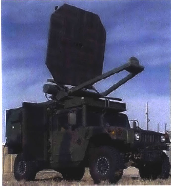
Figure 1-5: The U. S. Military Active Denial System, which operates at 95 GHz. A humvee is necessary to move the equipment.
