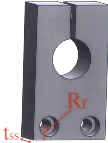
Figure 3-31: Shaft mount distances
