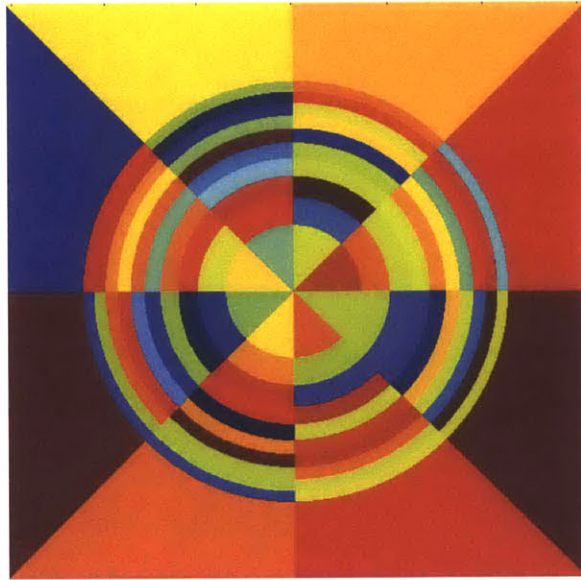
Figure 2-10: A pin-cell discretization with 8 azimuthal sectors and 10 equal volume radial rings.
