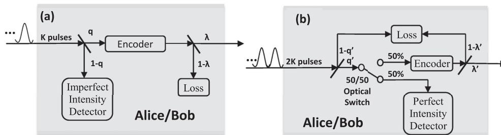
FIG. 3. (a) The actual model for Fig. 2. All the internal loss of Alice or Bob is modeled as a  $\lambda/(1-\lambda)$  beam splitter. (b) An equivalent virtual model. The loss is modeled as a  $\lambda'/(1-\lambda')$  beam splitter.  $q' = \eta_{\text{ID}}(1-q)$ , where  $\eta_{\text{ID}} \leq 1$  is the efficiency of the imperfect intensity detector.  $\lambda' = q\lambda/q'$ . The virtual model, which has features from (a), is used to analyze the security of (a).
