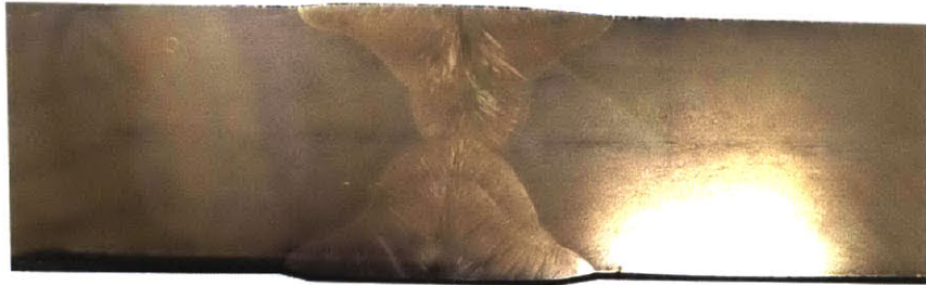
Figure 8: Weld sectioned sample after etching with Kalling's Reagent. The weld bead's shape can be seen with the added contrast.
