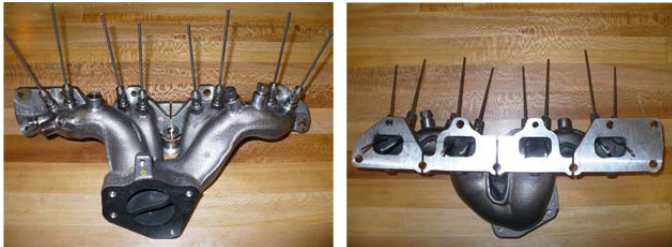
Figure 2. Secondary air injection hardware
