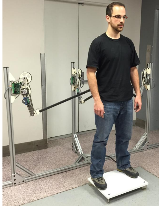
Figure 12. The six DOF modular parallel mechanism for unconstrained human motion. Three actuators can redundantly generate force on the transverse plane.
