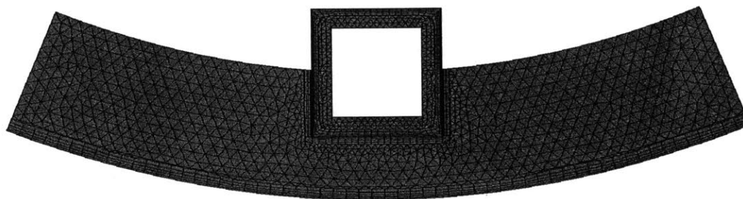
Figure 6.2 Illustrated mesh of the model domain. (The actual mesh used in simulation is much finer.)
