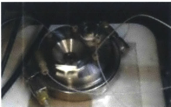
Figure 52. Image of first-generation Nanofiltration module assembled for operation.
