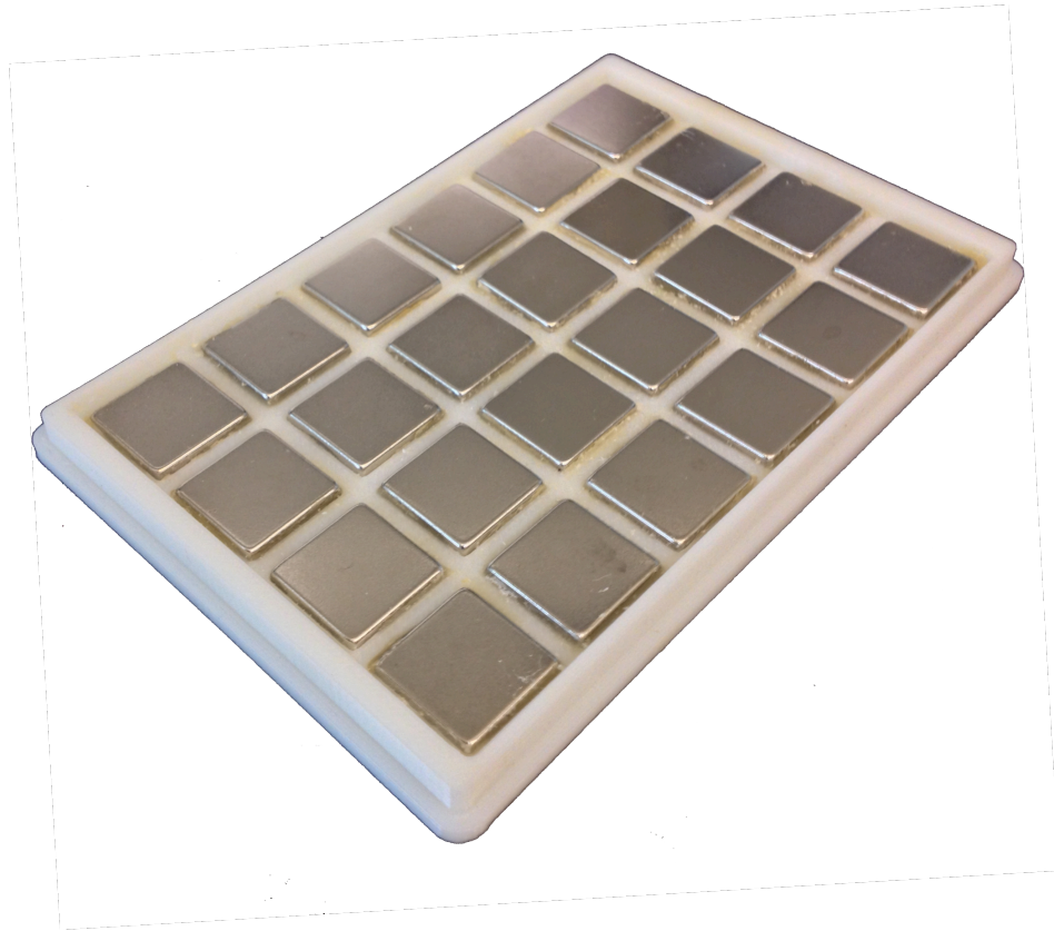
Figure 31. Magnetic plate (MagPlate) for CTC enrichment.
