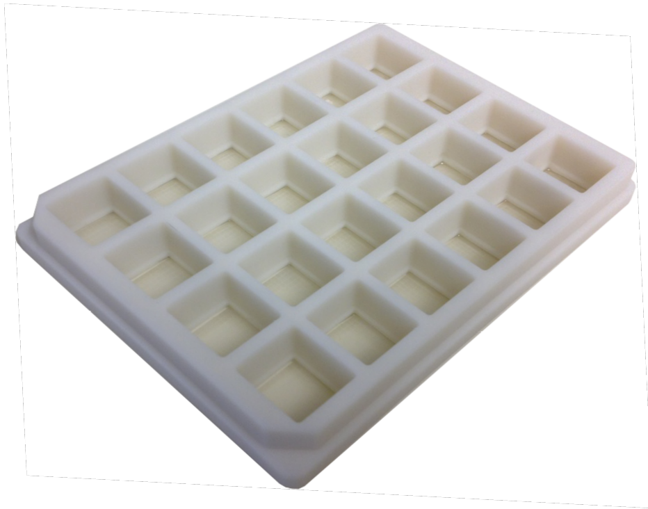
Figure 24. Nanowell plate for single-cell cytometry.
