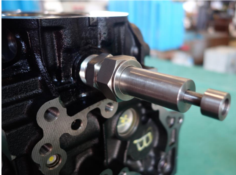
Figure 4-13. LIF Focusing Probe Installation into Engine Block via NPT Fitting
