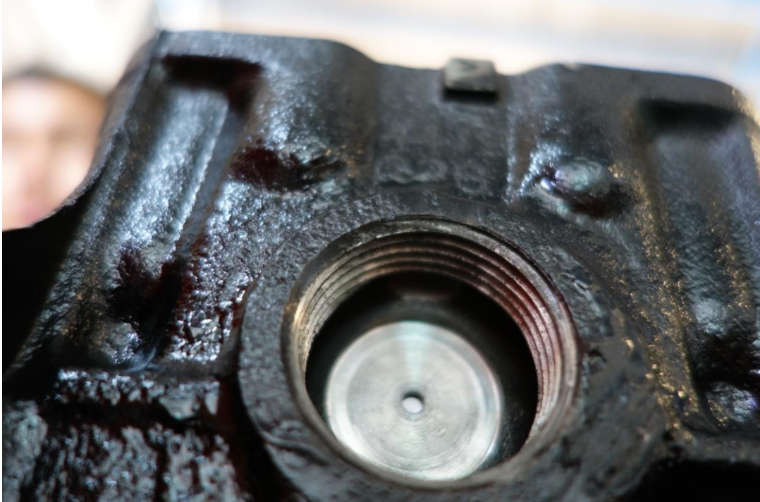
Threaded tunnel bored through the engine block
