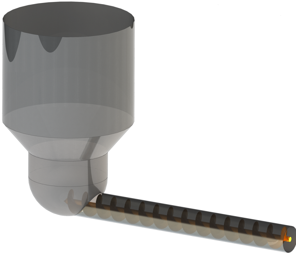
Figure 3-2: A Computer-Aided Design (CAD) model of the hopper and auger used in the ISRU system model.
