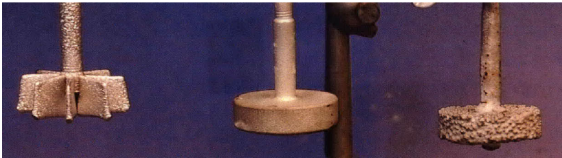
Figure 1-3: Three different anodes tested by Paramore [79], created by coating graphite geometries with iridium via electrodeposition.
