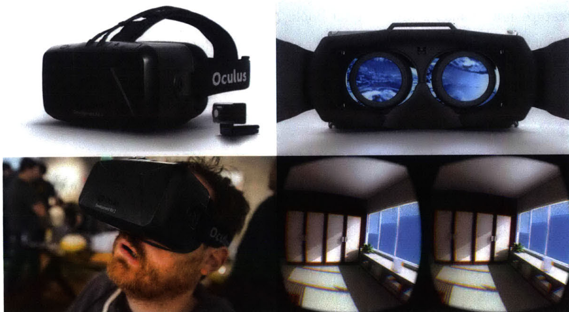
Figure 3-2: Oculus Rift DK2 and an example of the display (bottom right)
