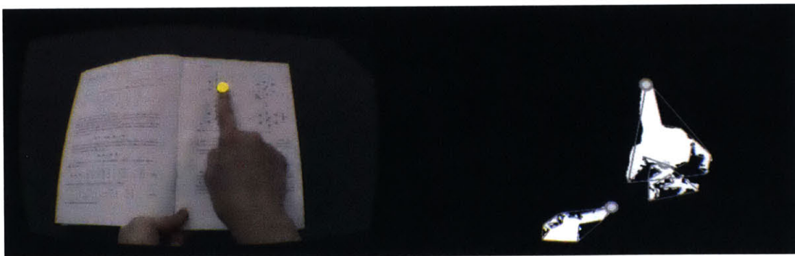
Figure 3-8: RGB camera view (left) and the thresholded image of the hand mask (right)
