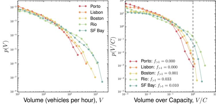
Figure 5-4: Distributions of travel volume assigned to a road and the volume-over-capacity ( $V/C$ ) ratio for the five cities. The values presented in the legend refers to the fraction of road segments with  $V/C > 1$ .
