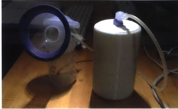
Figure 11: Completed breast pump showing the white cylindrical enclosure and collection flange and bottle from an off-the-shelf pump.
