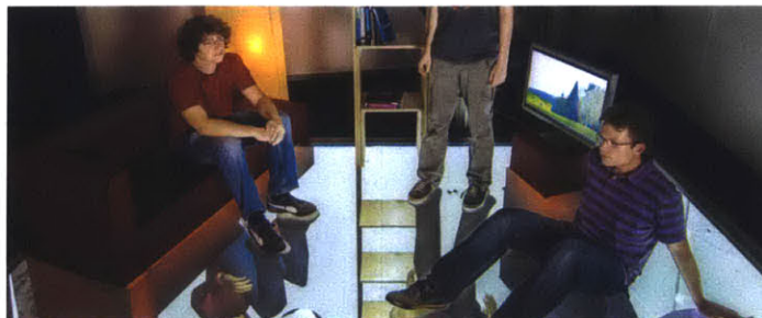
Figure 28: Students sitting on the GravitySpace prototype demonstrating the systems ability to recognize objects and project a digital mirror-image in those positions. Image Source: Hasso-Plattner-Institute
