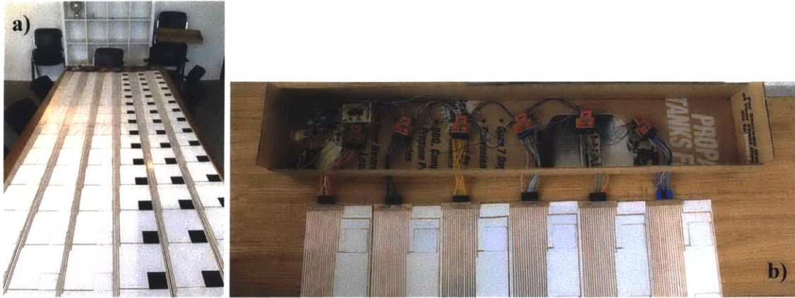
Figure 48: a) View of the six-strip prototype assembly. Note half the FSRs do not have a square of paper yet. b) View of the electronics connected to the strips.
