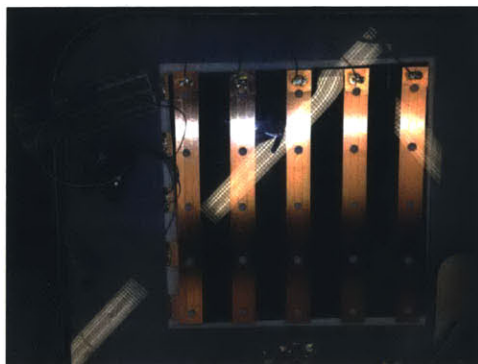
Figure 37: Smaller pressure mat prototype with 25 sensors (white dots indicate location).
