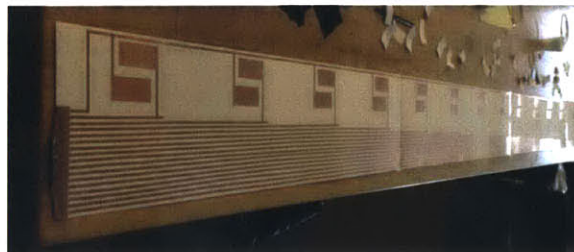
Figure 47: One sensing strip with pads at each FSR location.
