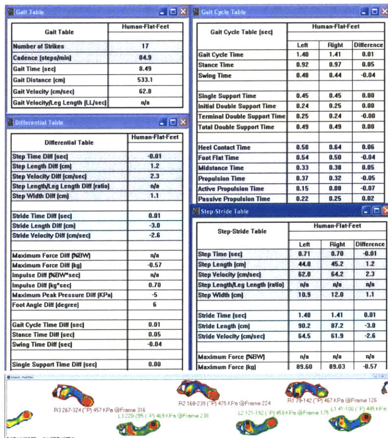
Figure 118: Pressure output and gait cycle analysis by Tekscan Walkway™ gait analysis system. Image Source: Tekscan
