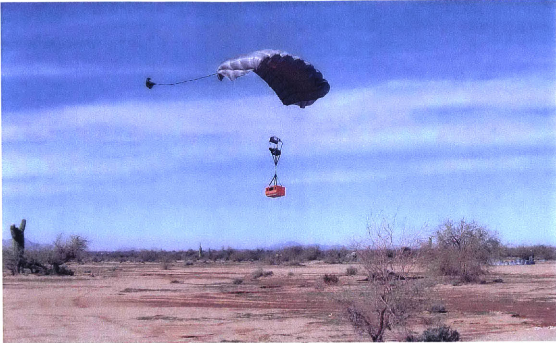
Figure 6-3: Deployed UltraFly parafoil system with MC-5 canopy during flare at Eloy test range (author photo)
