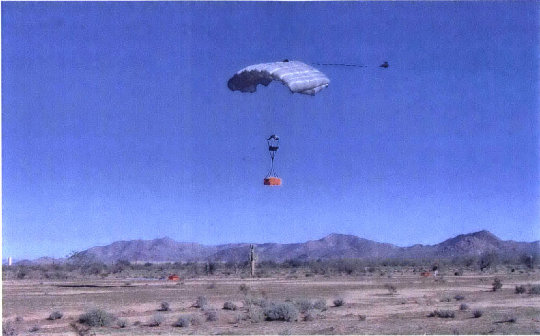
Figure 1-2: Autonomously guided UltraFly parafoil system (author photo)
