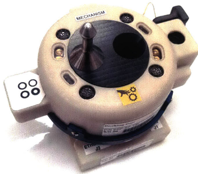
Figure 3-1: The Final Flight Design of the SPHERES Universal Docking Port
