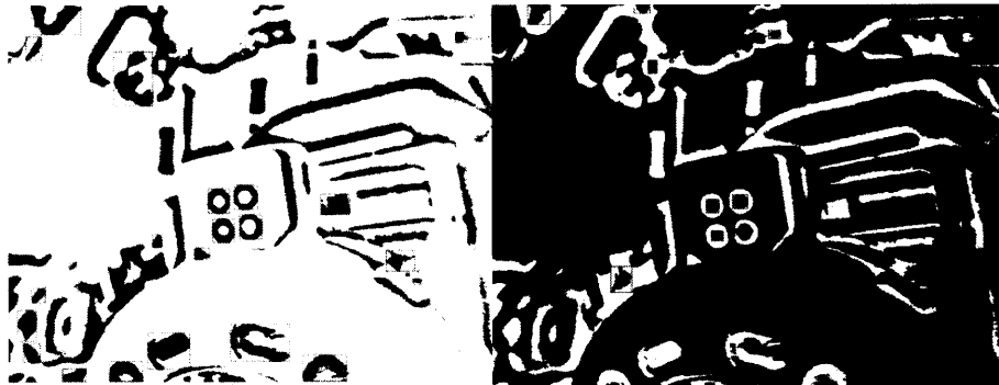
Figure 4-7: The Result of Performing Adaptive Thresholding on a Grayscale Image and Its Inverse
