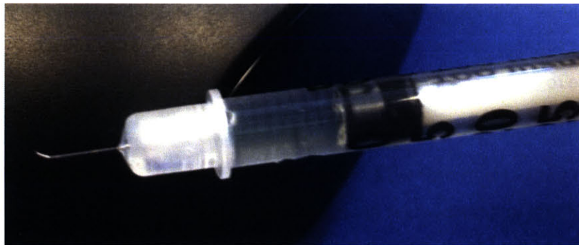
Figure 5.5 Image of the needle modification that was made to the insulin syringe for the intrathecal injections.
