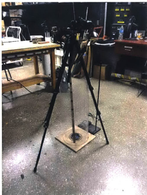
Figure 28: This image shows the set-up for the birds-eye view method discussed in Section 2.3.3.1 . The camera is positioned looking down at a cross-section of the flow mixing, while the laser illuminates a slice of the flow. In this set-up, the inner cylinder is not in place in the mixer, as it was a set-up for test images. However, the laser and camera position will remain as pictured here for image collection using the final assembly.
