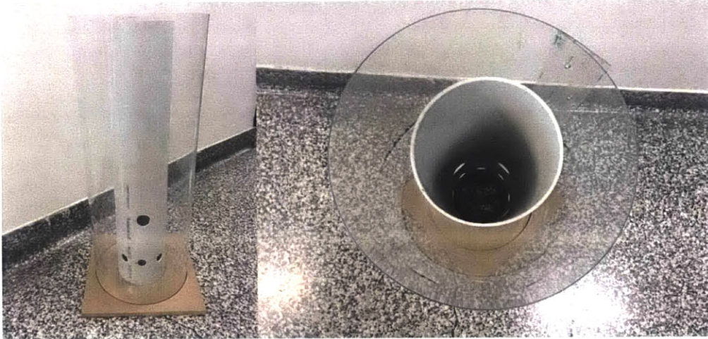
Figure 7: These images show a side view and a top view of the nested cylinders which were machined for this project. The cylinders are press fit into the grooves that are cut into the MDF to prevent cylinder movement during imaging processes.
