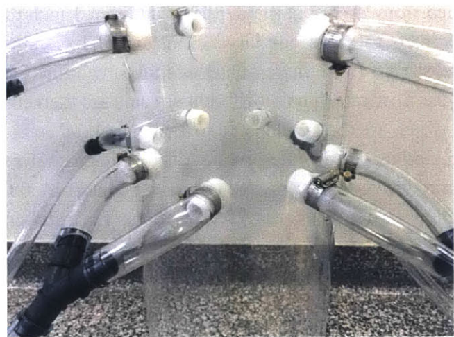
Figure 21: The assembled inlet system for the primary and secondary outlets for the outer cylinder is shown here.
