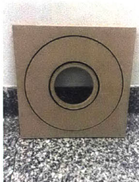
Figure 6: The base for cylinder alignment consists is machined out of 5/8-inch MDF. The channels are is 3/8-inch deep and the hollow center allows air lines to be routed to the inlets on
