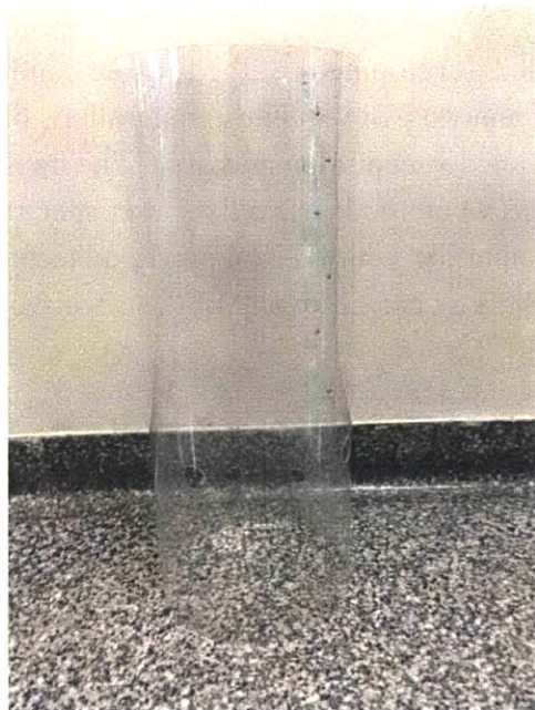
Figure 4: The outer cylinder is constructed out of 1/16-inch PETG bent into a circle and held in shape with pop rivets. There are four 1-inch diameter primary inlets and eight 1-1/2-inch secondary inlets waterjetted in the part. Please note that the design pictured here has 8 primary inlets and 4 secondary inlets. For imaging, only 4 of the primary inlets are used. The remaining
