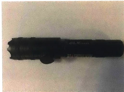
Figure 23: A Barska GLX green 5mW Tactical Laser Sight was used as the light source for the laser line.
