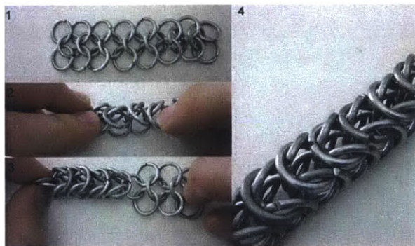
Figure 2.3: 2.3.1 shows the European four-in-one weave, which, when manipulated as shown in 2.3.2 and 2.3.3, will create the box weave shown in 2.3.4. The box weave will behave like a cylindrical sample of the European four-in-one weave. [7]
