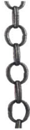
Figure 2.1: A chain weave is characterized by each ring passing through two other rings. [5]
