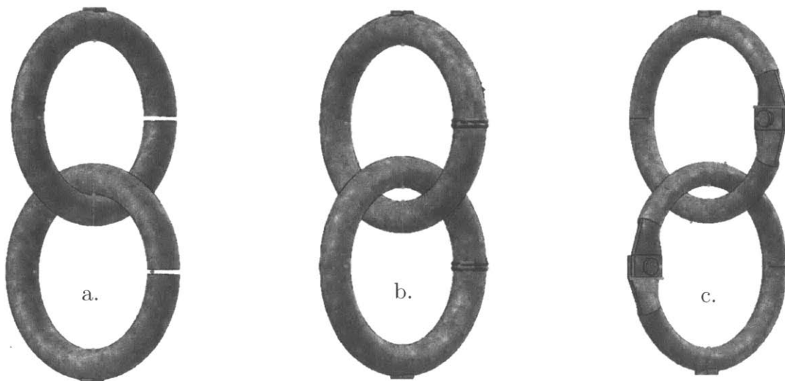
Figure 3.3: SolidWorks models created for simulating butted, riveted, and welded rings. The splits, welds, and rivets were all oriented at 90^\circ angles from the vertical, as this position is in the middle of the range of possible positions for these features. (a) Depicts a chain of 12-gauge, D2 rings with a gap size of 0.3 mm. (b) Depicts a set of welded 12-gauge, D2 rings with the weld 0.6 mm in width. (c) Depicts 14-gauge, D3 riveted rings with a rivet diameter of 0.7 mm.
