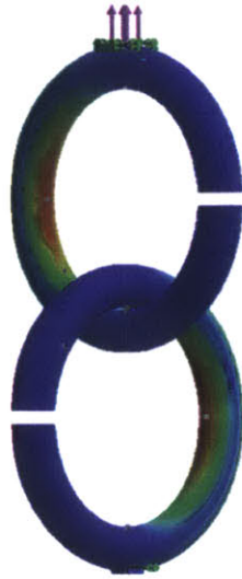
Figure 8.1: Image of the stress profile in the rings generated by a SolidWorks simulation of 12-gauge, D2 butted rings with a 0.3mm gap at the 90° position. Stress is concentrated at the fixed feature at the bottom, the feature that the force was applied to at the top, and in the middle of the bend in the ring. Additionally, very little force is experienced by the side of the ring with a split in it.
