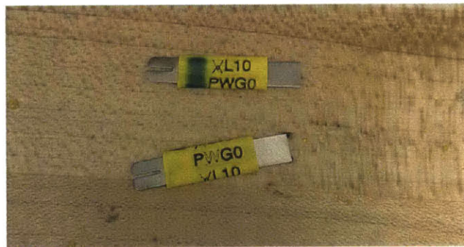
Figure 3-7: 1A-2.5A resettable circuit protectors used to connect negative cell terminals in 5p configuration
