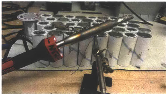
Figure 3-4: Large soldering iron used for tinning large positive contacts
