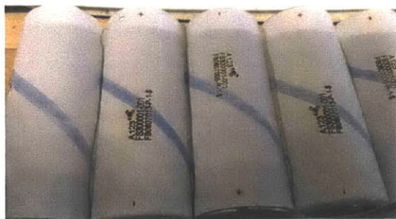
Figure 3-2: Five cells glued in parallel, yielding 5p configuration
