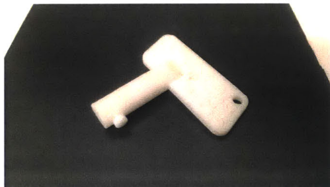
Figure 4-3: 3D-printed Hella battery master switch key
