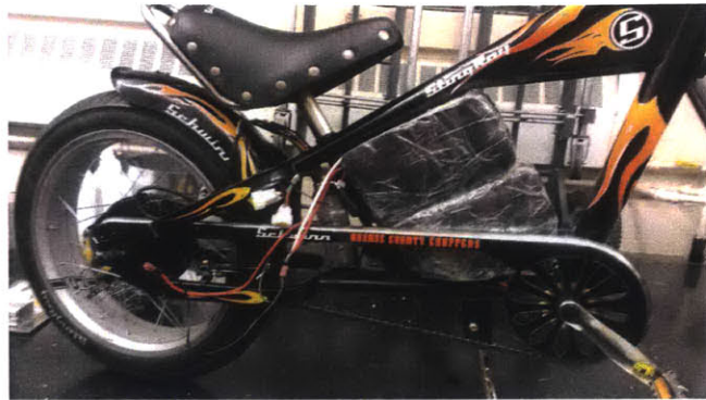
Figure 4-1: Controller and battery pack placement within bicycle frame
