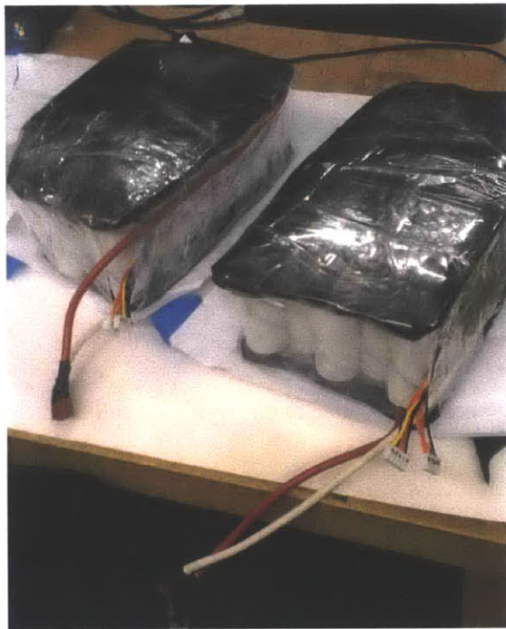
Figure 3-11: Battery packs wrapped with clear packing tape to secure foam and cell alignment, and to protect power and balance wires from fatigue
