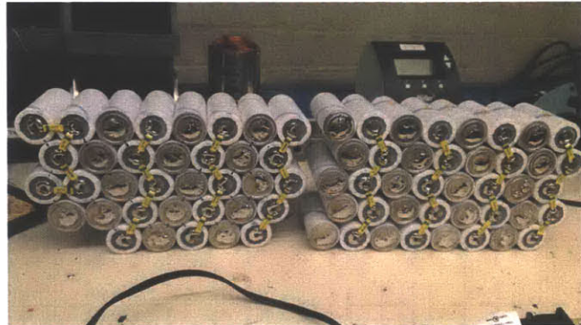
Figure 3-8: All negative terminals connected with circuit protectors and solder
