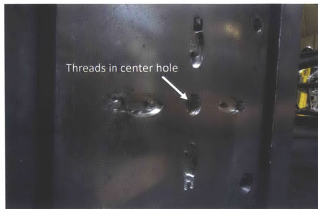
Figure 3-8: The core side with threads in the center hole. Photograph by author.
