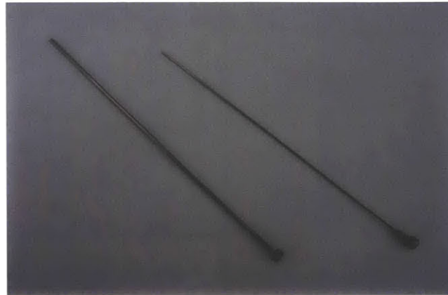
Figure 3-10: Ejector pins shown above with the 3/32" on the left and the 0.043" shoulder pin on the right. Photograph by author.
