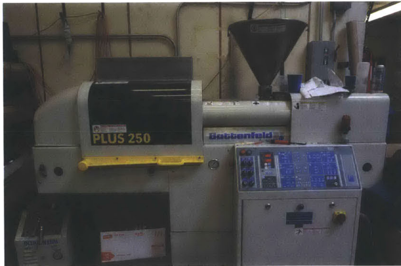
Figure 4-1: The Battenfeld PLUS 250 Unilog 1020 in Area 51. Photograph by author.
