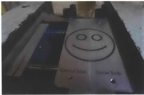
(a) No gap between MUD frames
