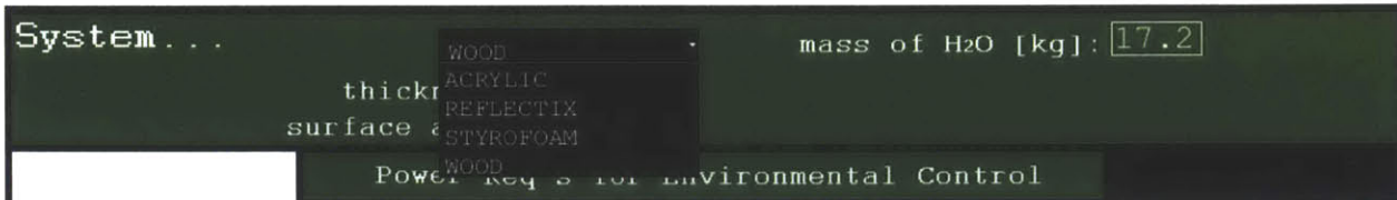
Figure 3-11: A drop-down list displays material choices for the GRObot jacket outer. Each material is associated with its thermal conductivity, which is used to update R_{lower} .
