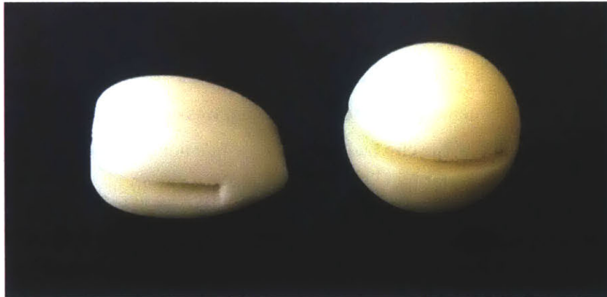
Figure 16. Clips with more rigidity were better able to hold onto the battery. Also, a simplistic design allowed for artistic interpretation when integrated into the circuits.
