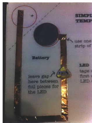
Figure 2. Circuit with battery placement.
