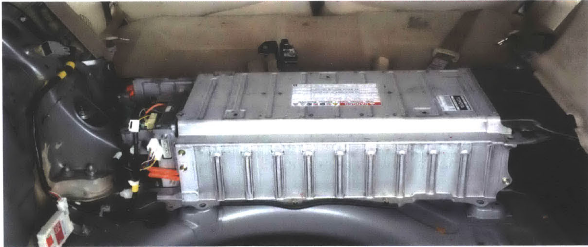
Figure 1: The nickel-metal hydride battery pack from a Toyota Prius. The battery has a nominal capacity of 4.4 kWh and weighs around 110 pounds (source: forbes.com)
