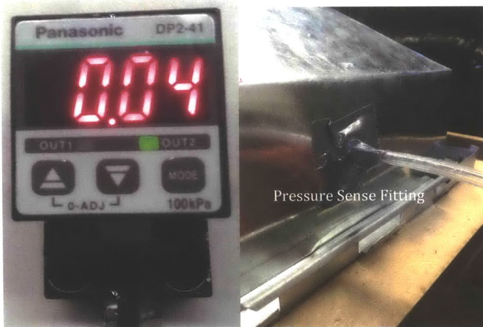
Figure 19: The manometer used for measuring airflow over the test and the place in the duct system where the pressure was measured
