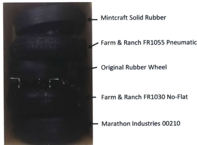
Figure 22: Top view of wheels which were tested under compression.
