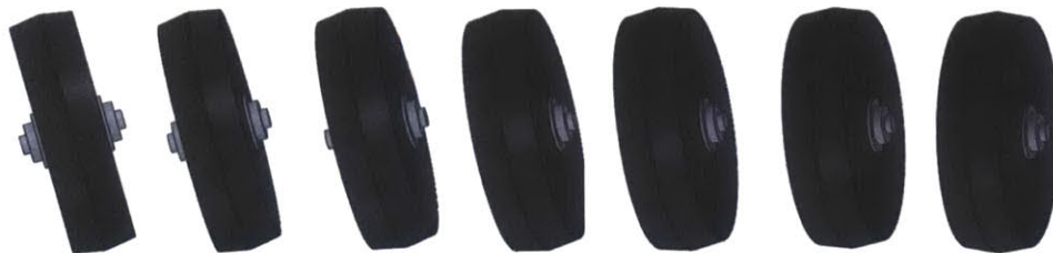
Figure 8: Visual of hub misalignment causing the tire and wheel to not be square.
