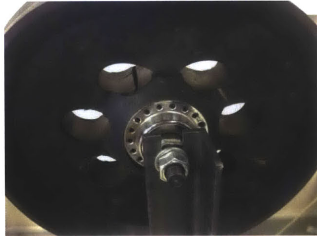
Figure 20: Visible crack in rubber of the original wheel caused by a 5,000N compressive load.
