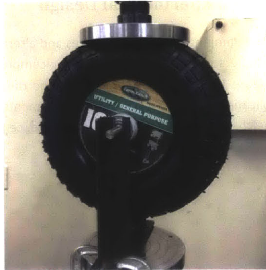
Figure 19: Fixturing set-up for Instron compression testing of wheel.
