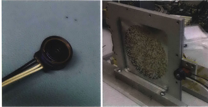
Figure 3-8: TiNi SW04 Switch washer (left) and its placement in the Frangibolt stackup of the EM Radiation Cover subassembly
