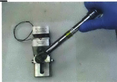
Figure B-3: Compression of Frangibolt [7]
