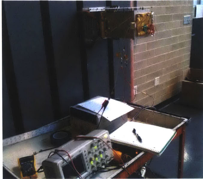
Figure 3-6: REXIS spectrometer horizontally mounted on a wall during a Frangibolt actuation. A functional CCD is present within to determine if the shock from the actuation and Cover deployment will damage the detector.
