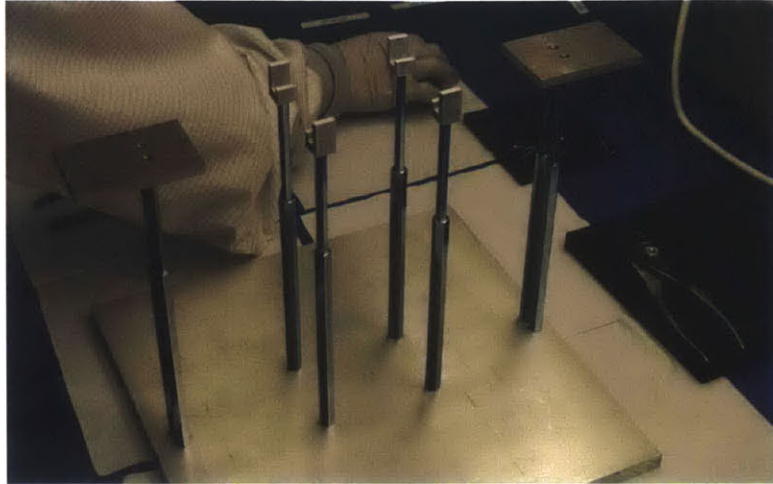
Figure 4-12: Assembly jig used during the DAM assembly
