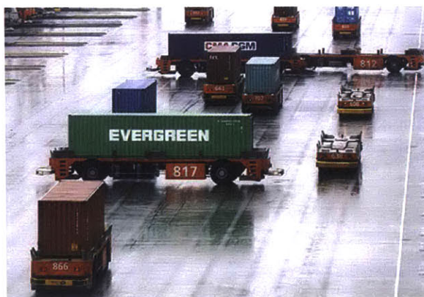
Figure 1-2: Unmanned automated guided vehicles (AGV) transporting containers in Europe’s largest sea port, in Rotterdam, Netherlands [30].
