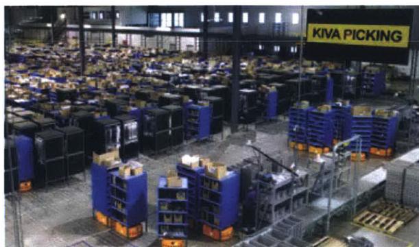
Figure 1-1: A warehouse populated with Kiva Systems LLC robots, automating warehouse logistics [10].
