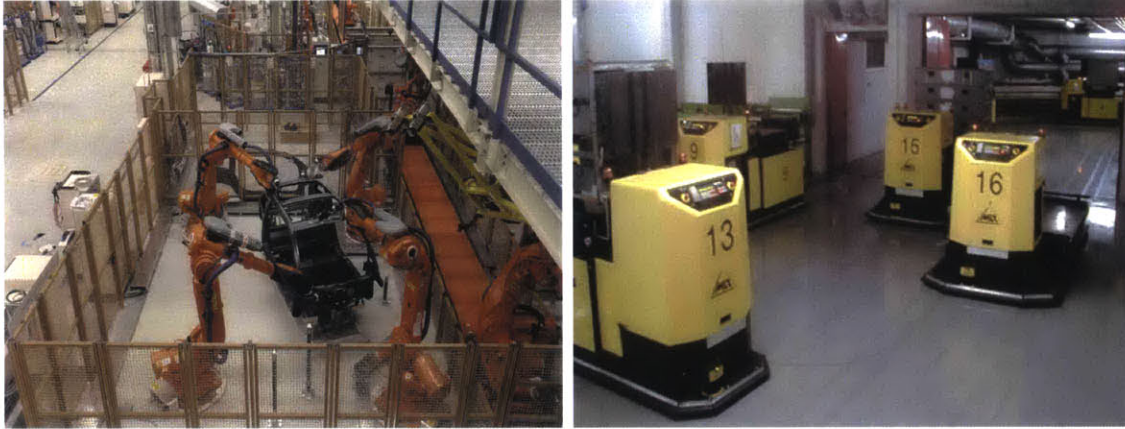
(a) Large, industrial robots performing the initial phase of car manufacturing. [5] (b) Automated guided vehicles delivering parts in an automotive assembly line. [3]
