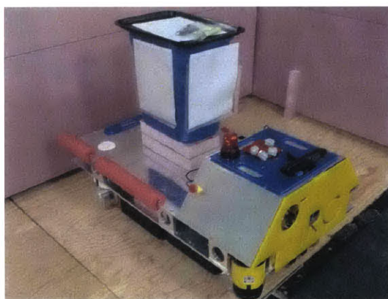
Figure 4-2: The Rob@Work mobile robotic platform augmented with additional sensors, a raised platform and tray. The modified setup is used as the robotic assistant for human subject experimentation.
