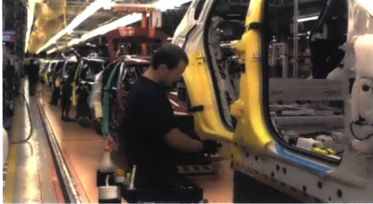
Figure 1-2: A typical, final automotive assembly line [10]. The assembly line includes human associates, dynamic objects such as part-carts, and a conveyor belt which ferries the cars that are being assembled. The human associates primarily work on the conveyor belt, and periodically ferry tools and parts from outside the conveyor belt to carry out the car assembly.
