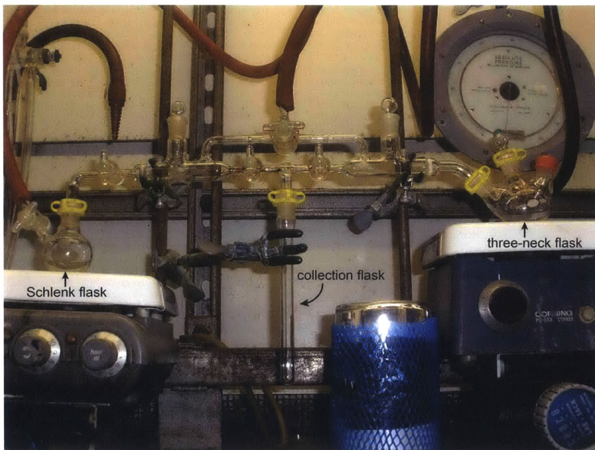
Figure 9-20: Apparatus for the synthesis of ^{15}\text{NO} .
