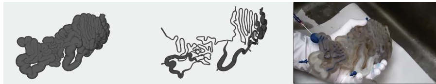
Figure 14: Second small-scale support test. Left: 3D test geometry. Center: Inner channel geometry (STL). Right: Testing model that was supported using liquid support. Image courtesy of Tal Ely & Daniel Divovsky of Stratasys.
