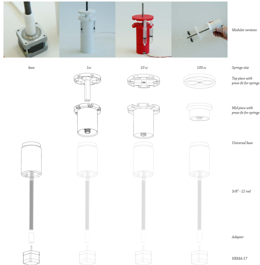
Figure 33: Modular 3D printed components of the syringe pump. (A) The base of the pump which includes the Nema 17 stepper motor, a 3D printed connector, and the 3D printed base. The motor press fits into the 3D printed base. (B) The components for a 1cc syringe pump, the pump used to run the gene assemblies. The Mid piece, above the base components, screws into the base. The Top piece is threaded and is moved vertically by the threaded rod. (C) The Mid & Top pieces were modified to accommodate 10cc syringes. (D) The Mid & Top pieces were modified to accommodate 100cc syringes. Photo credit (top images): Che-Wei Wang and Taylor Levy
