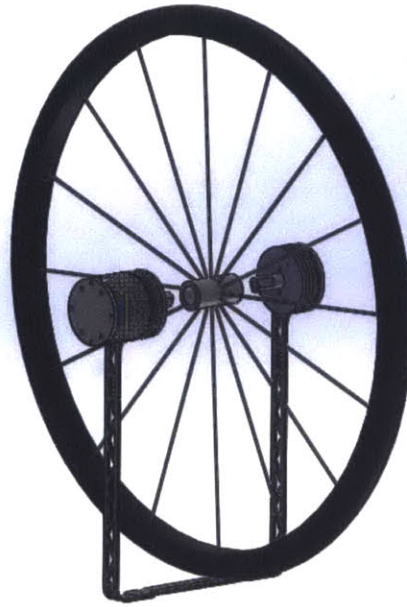
Figure 3-2: A CAD representation of the system in relation to a bicycle wheel.
