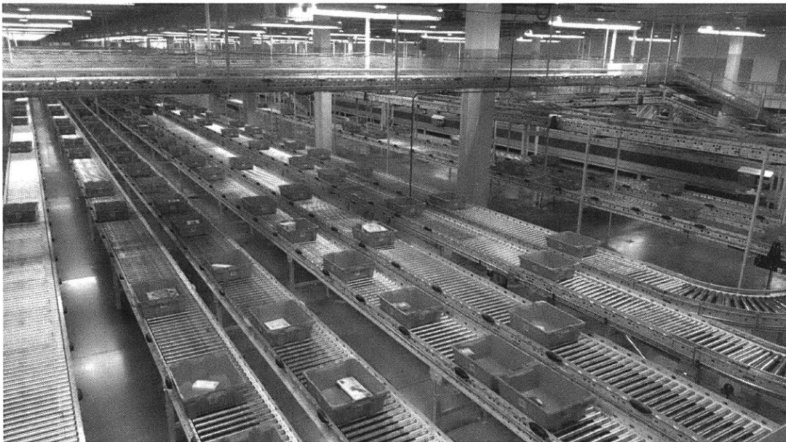
Figure 2-1: Conveyance, trays, and items in an automated material handling system
