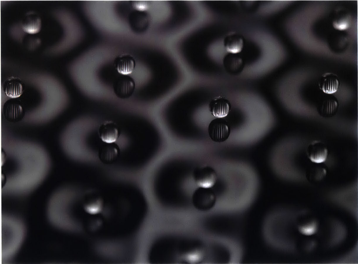
Figure 2-19: A stable lattice of oil droplets, formed with our droplet generator, bounces on the surface of a vibrated oil bath.
