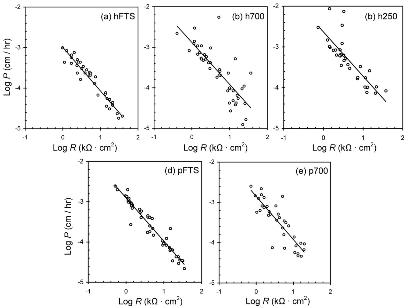
**Fig. 1.** Comparison of the experimental  $\log P - \log R$  correlations: (a) hFTS,  $n = 36$ , (b) h700,  $n = 44$ , (c) h250,  $n = 34$ , (d) pFTS,  $n = 47$ , and (e) p700,  $n = 35$ . Each data point represents one experiment. The solid lines represent the linear regressions fitted to each data set. The statistical parameters associated with the linear regressions are listed in Table 1.
