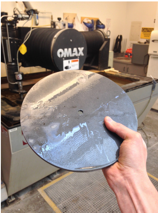
Fig. 4.2.14: Waterjetting steel cap for end-node.
