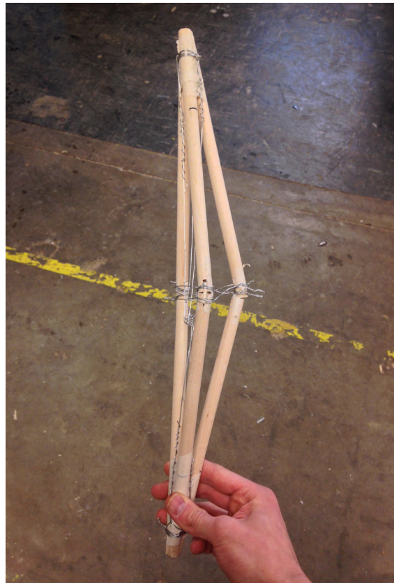
Fig. 4.2.7: Global buckling failure.
