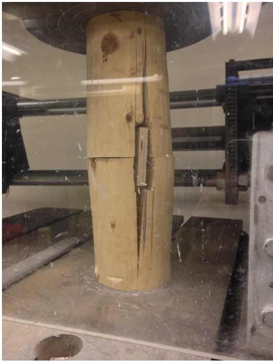
Fig. 4.2.3: Initiation of splitting failure in compression-only connection.
