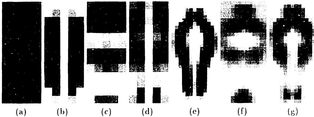
Figure 6-17: Ensemble average values of the wavelet coefficients coded using gray level. Coefficients whose values are above the template average are darker, those below the average are lighter. (a) vertical coefficients of random scenes. (b)-(d) vertical, horizontal and corner coefficients of scale 32 \times 32 of images of people. (e)-(g) vertical, horizontal and corner coefficients of scale 16 \times 16 of images of people.
