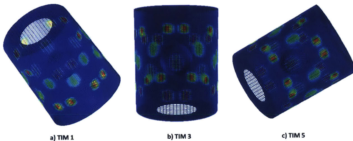
Figure E.4. WRF views of the hohlraum and implosion from a) TIM1, b) TIM3, and c) TIM5, for the 2-cone implosions performed on Sept. 1st 2011. Color indicates the total energy deposition on the inside of the hohlraum wall by the lasers. The protons observed from the TIM1 line-of-sight pass between two laser spots, and may experience scattering in the buildup of gold plasma from the colliding plasma bubbles. The protons observed from TIM3 and TIM5 pass directly through the center of a laser spot, and will tend to be concentrated by the magnetic field structure of the plasma bubble.
