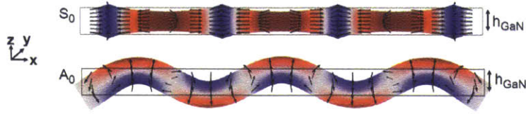
Figure 5-1: Cross-section of an infinite plate of finite thickness, h_{\text{GaN}} shows the first two Lamb modes propagating in the x -direction. The zeroth order symmetric Mode, S_0 , is shown for a normalized wavelength \lambda/2d = 4.3 . The mode shape of the zeroth order antisymmetric mode, A_0 is shown for a normalized wavelength \lambda/2d = 6 . Arrows represent the displacement fields, while the color maps the strain fields.
