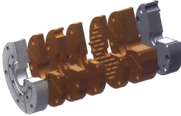
Figure 6-1: Expanded three quarter section view of the solid model of the 17 GHz PBG structure, showing two coupling cells and central PBG cell. The coupling rods are not shown for clarity. Power is coupled in from the left.
