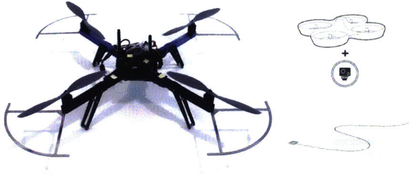
Figure 10. Early prototype of the Aerial Quadcopter built to perform hyper-spectral imaging (left). The S-shape route of the lead vehicle above the Charles River (right) (Illustration Credit: Chris Green, Technical Submission to the UAE Drones For Good Competition. Dec 1, 2014)
