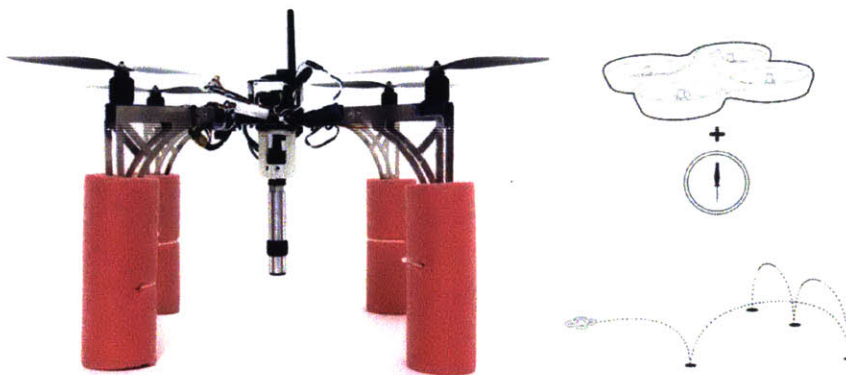
Figure 11. Early prototype of the 3DR Aerial Sampling Quadcopter (left) Sketch of the type of route on which the probing vehicle s move (right) (Illustration Credit: Chris Green , Technical Submission to the UAE Drones for Good Competition. Dec 1, 2014)
