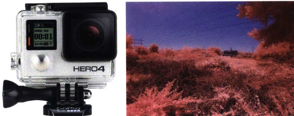
Figure 13. GoPro camera with infra-blue lens fitted (left) Example of infrared images returned by camera (right) (Photo Credits: Chris Green, Technical Submission to the UAE Drones For Good Competition. Dec 1, 2014)
