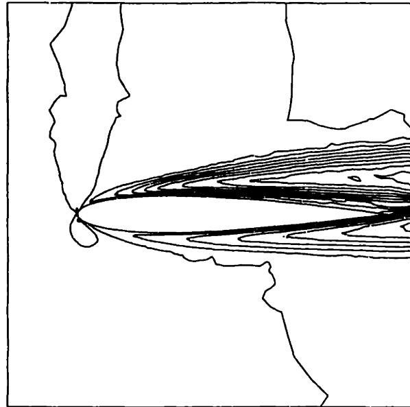
Figure 3-23: \partial \rho u / \partial \alpha distribution for NACA0012, Re=2000 , M_\infty = 0.8 , \alpha = 3.5 deg (Scheme II) from finite difference with \Delta\alpha = 0.01
