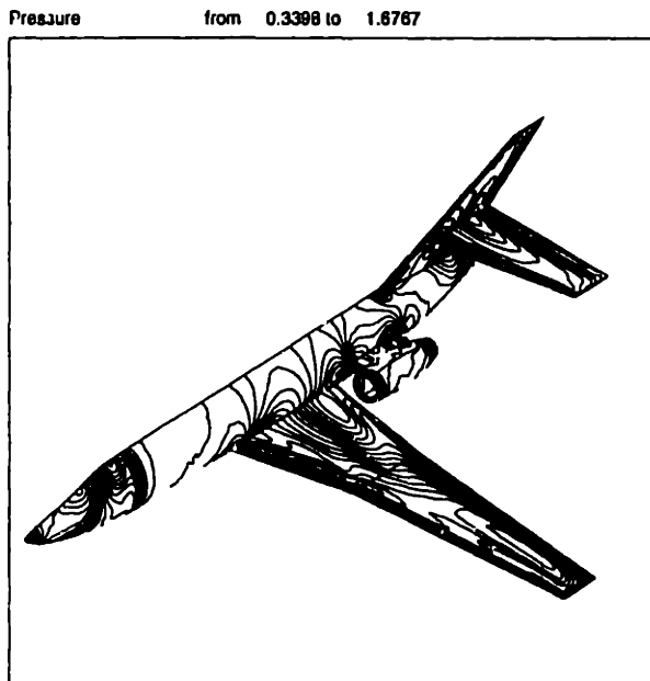
Figure 4-19: Baseline surface pressure contours for business jet at M=0.85 , \alpha = 2^\circ
