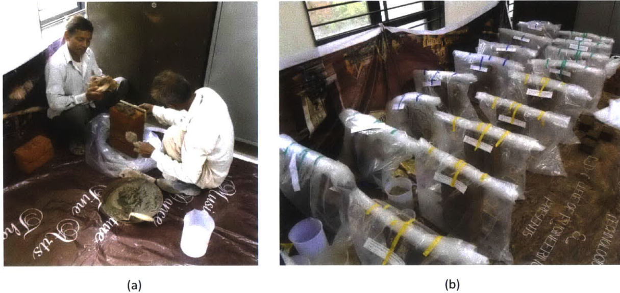
Fig. C.5. Masons constructing prisms (a) and completed prisms in the curing process (b).
