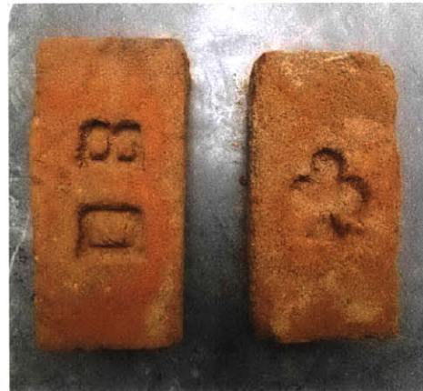
Fig. C.2. A high strength brick (left) and a low strength brick (right).
