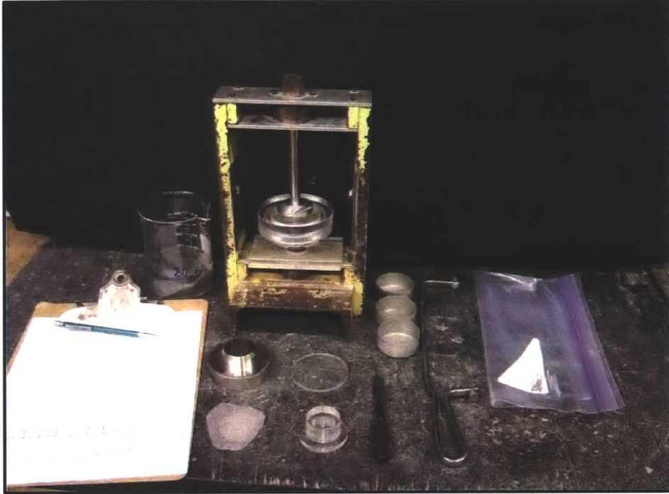
Figure 5-3: The trimming and vertically-draining CRS set-up equipment is laid out and prepared prior to sample extrusion.
