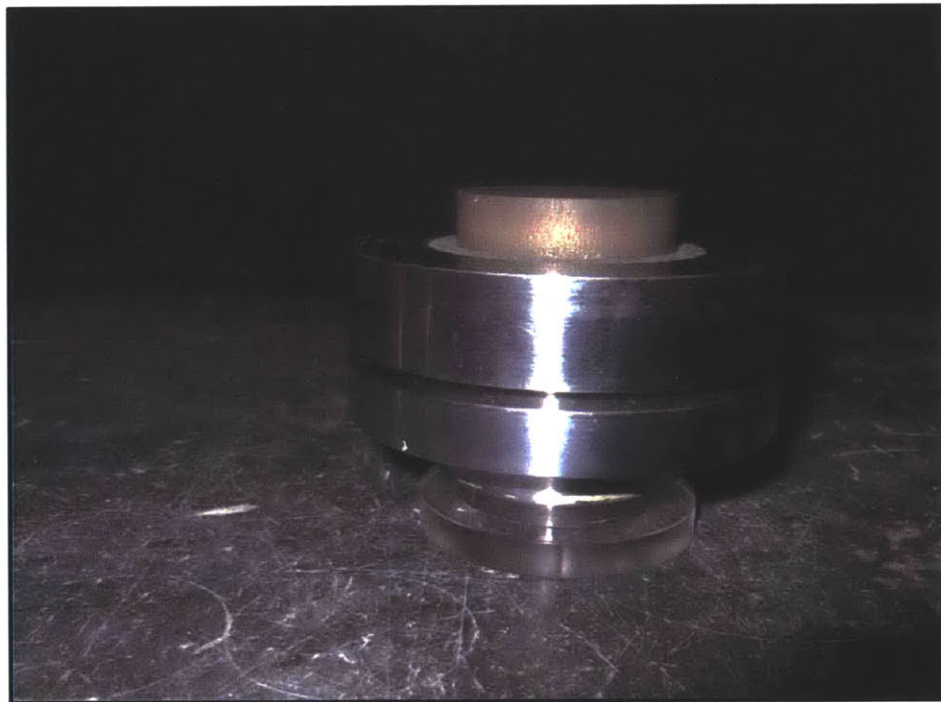
Figure 5-22: The cutting shoe and confinement ring are advanced to meet the shoulder of the acrylic spacer to transfer the specimen into the confinement ring and to set its height.
