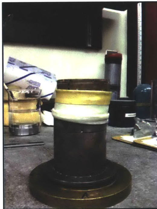
Figure 3-22: The coil-reinforced rubber membrane in concert with endcaps set to zero axial displacement create undrained horizontal simple shear in a DSS device. The profile of this sheared specimen (within the membrane) shows a parallelogram with non-right-angle corners.
