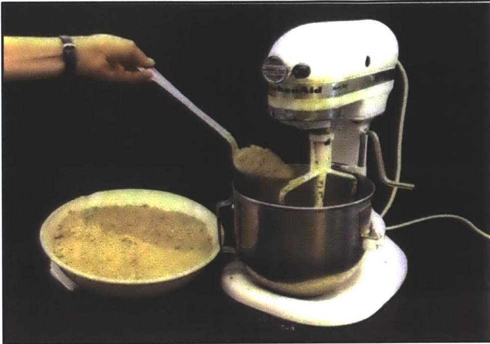
Figure 3-9: Soil powder is mixed into sea salt water using a Kitchen Aid® mixer (Casey, 2014).
