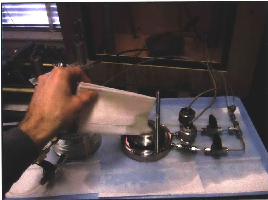
Figure 5-30: Paper towels can be used to absorb cell water when the cell is disassembled and to absorb water from above the specimen. Quick water absorption reduces specimen swelling.
