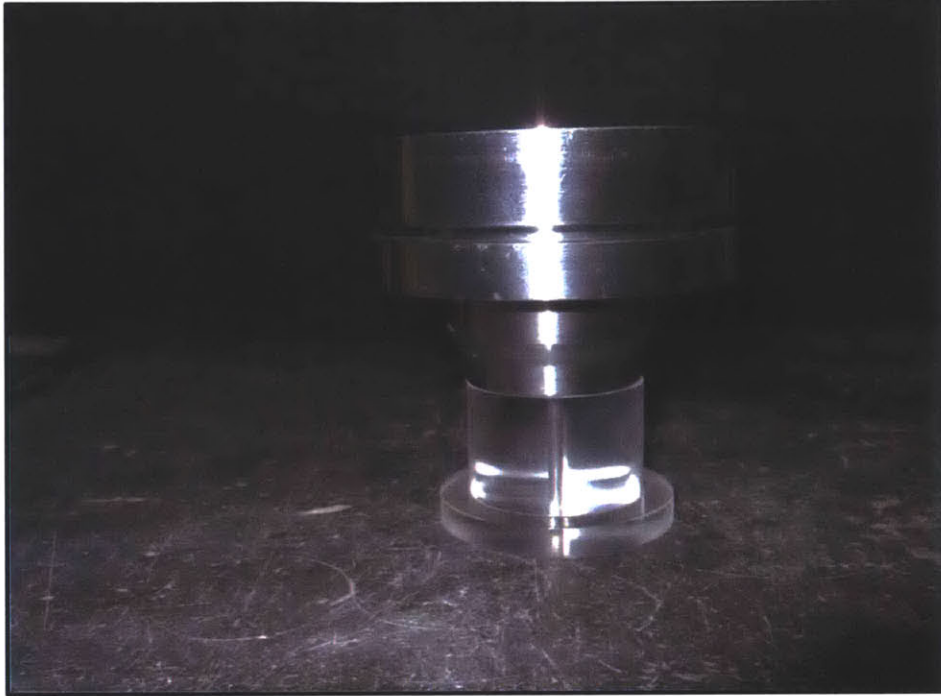
Figure 5-21: The confinement ring, cutting shoe, and specimen assembly is aligned with the top cap and acrylic spacer to transfer the specimen into the confinement ring.
