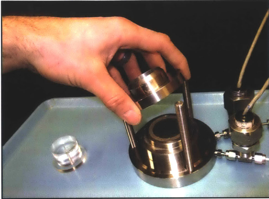
Figure 5-25: The acrylic spacer and cutting shoe are removed and the confinement ring, specimen, and top cap are left on the base for the duration of the CRS test.
