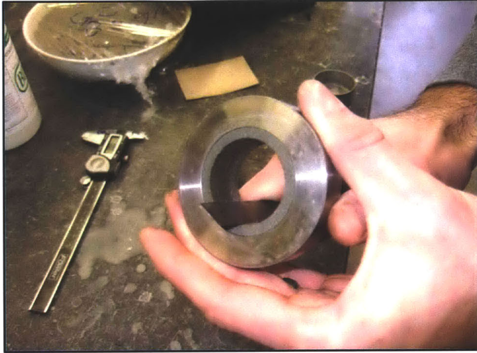
Figure 5-33: Extraneous soil should be collected from the confinement ring, top cap, and base pedestal after extrusion for a correct dry mass measurement.
