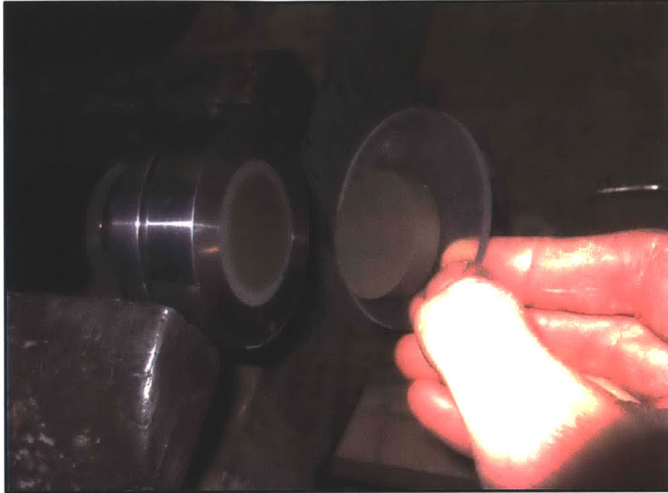
Figure 5-23: The bottom of the specimen is trimmed by placing the confinement ring, cutting shoe, specimen, top cap, and acrylic spacer assembly in a bench-mounted vice. The plastic disc aids in removing the trimmed soil.
