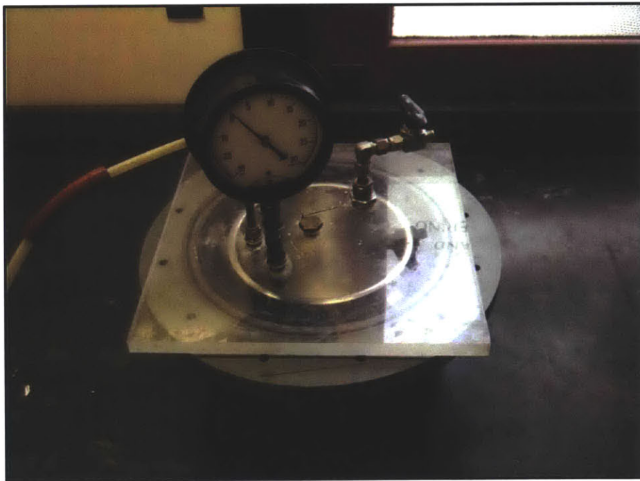
Figure 3-10: Soil slurry is evacuated in vacuum chamber under approximately 1 atmosphere of vacuum pressure for 20-30 minutes to removed entrapped air.
