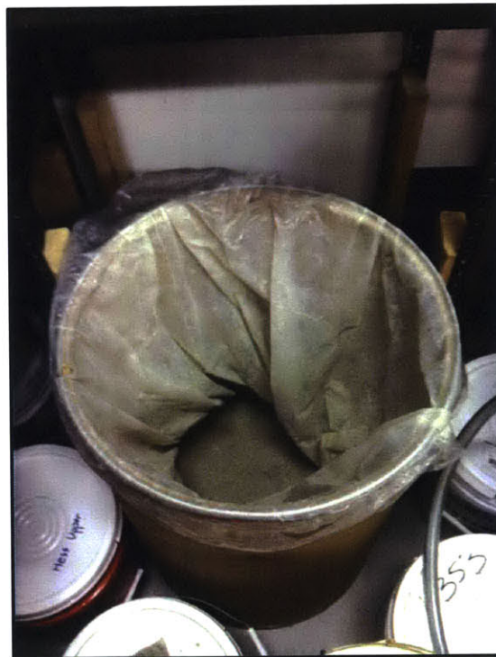
Figure 3-2: The BBC Series IV powder used has a grayish color and is stored in 40-gallon drums.
