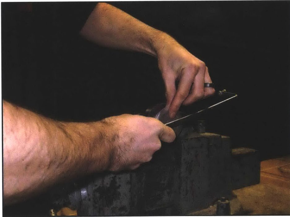
Figure 5-6: The top of the specimen is trimmed by placing the confinement ring in a bench-mounted vice. The wax paper aids in removing the trimmed soil.
