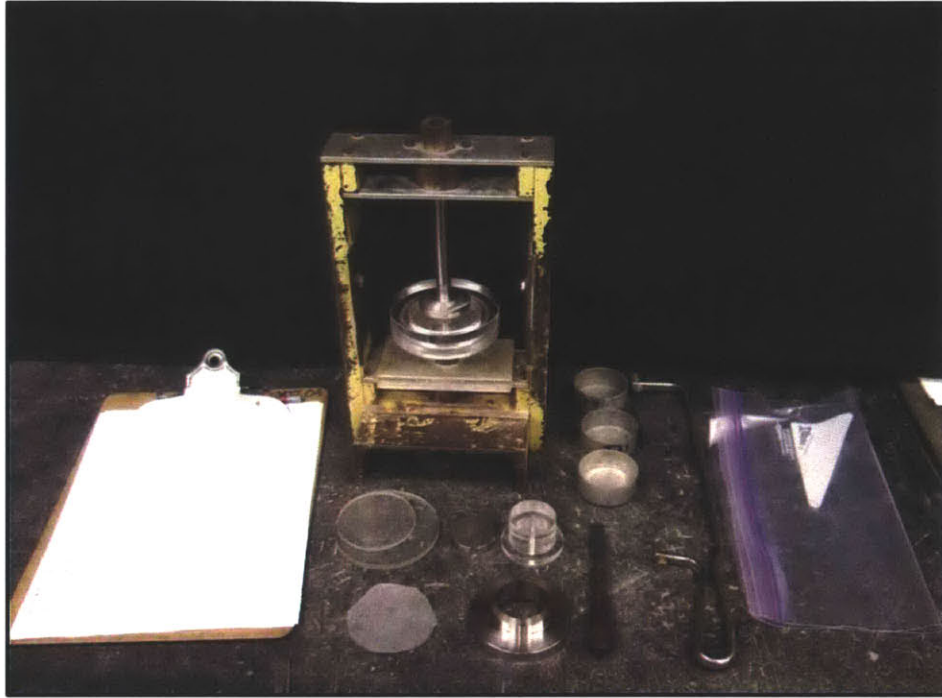
Figure 5-19: The trimming and radially-draining CRS set-up equipment is laid out and prepared prior to sample extrusion.
