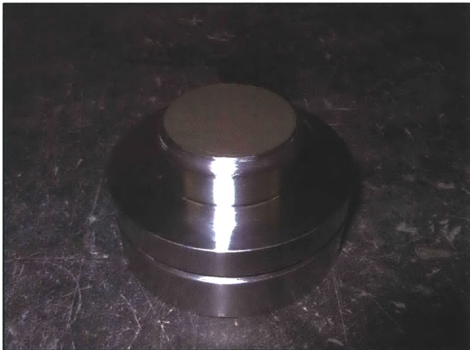
Figure 5-20: The cutting shoe is placed on top of the confinement ring to prepare for specimen transfer.
