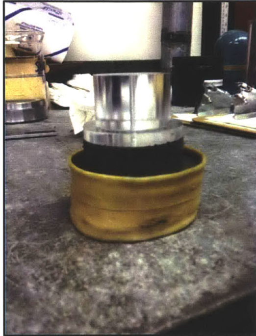
Figure 3-23: A smaller specimen is cored out of the larger specimen sheared in the DSS device using piano wire and acrylic cylinders as guides.
