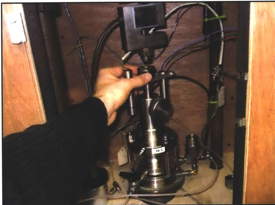
Figure 5-14: A moment/shear break is placed in-between the cell piston and the load cell on the load frame.
