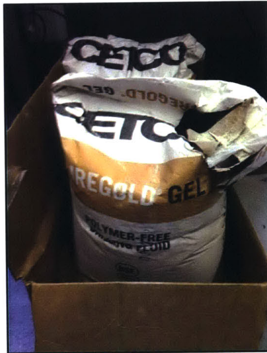
Figure 3-6: Puregold® Gel bentonite powder for drilling fluid is mixed with BBC to make BBC + 9% Mont. This is done in order to look at the effect of smectite (bentonite) content on mudrock permeability anisotropy.
