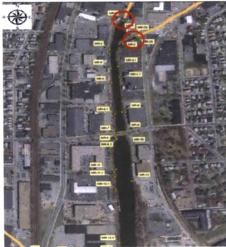
Figure 1-3: Malden River stormwater outfall locations. Source: (Nangle Associates 2014)
