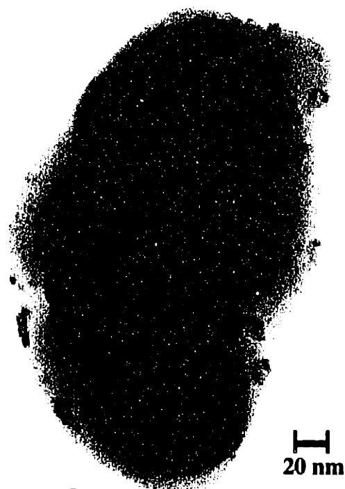
Figure 2.7. TEM micrograph of \text{Fe}_2\text{O}_3 /sulfonated- \text{SiO}_2 nanocomposite calcined at 500 °C under \text{O}_2 .
