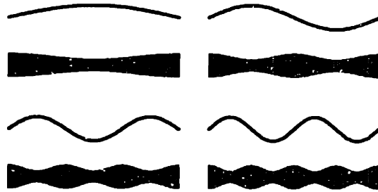
Figure 7.2 mode shapes and corresponding shape changes for a shaft with fixed ends
