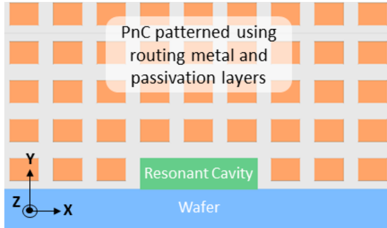
Figure 4-2: Cross-section schematic of a standard CMOS stack showing phononic crystal formed using BEOL layers, encapsulating resonant cavity formed in FEOL layers.
