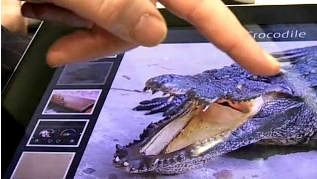
Figure 1-7: An image of Fujitsu Sensory Haptic Tablet Device. This tablet uses ultrasonic vibrations to convey tactile information by changing the friction between fingertips of a user and touch panel.
