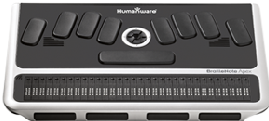
Figure 1-3: An image of Braille Notetaker device. This device has 32, 8-dot Braille cells for reading braille characters. This device can also act as keyboard for interacting with a PC. The cost of this device is $5,495.00.
