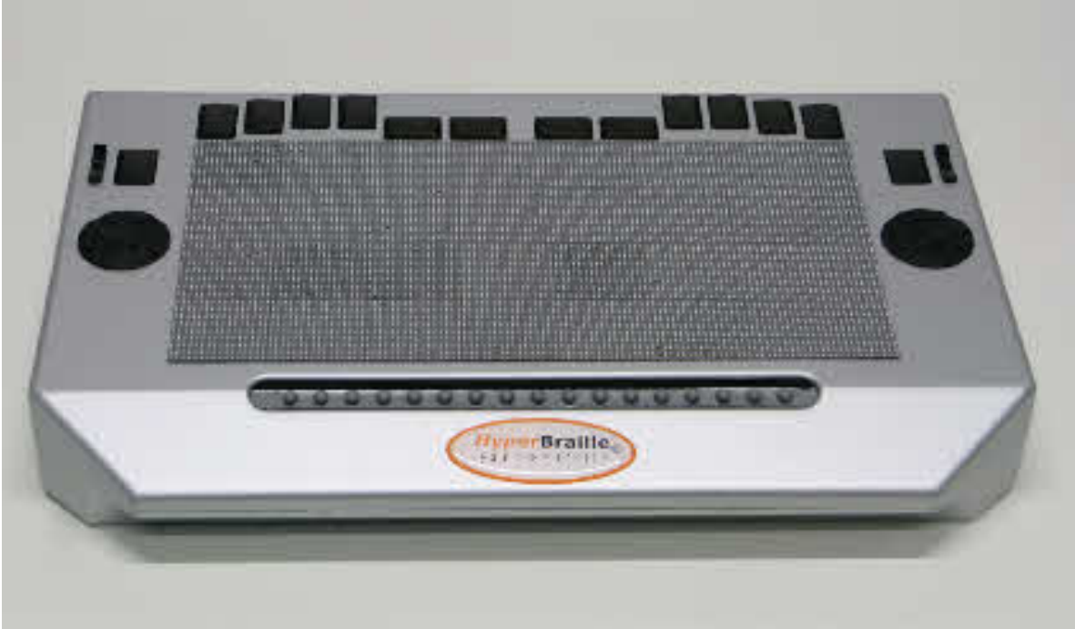
Figure 1-2: An image of the full page display of Metec-AG. This Braille device has 120 \times 60 = 7200 piezoelectric pins. These piezoelectric pins can vibrate in real time providing for fast graphical renderings. This hyperBraille device can also accept touch inputs from user's fingertips. But the device costs 45,000 euros which is huge drawback.
