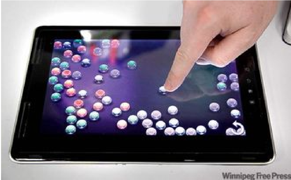
Figure 1-8: An image of the Senseg Tablet. This tablet uses an electrostatic field to create an attractive force between the touch-screen surface and the user's fingertips. By modulating this attractive force, the device provides various touch illusions.
