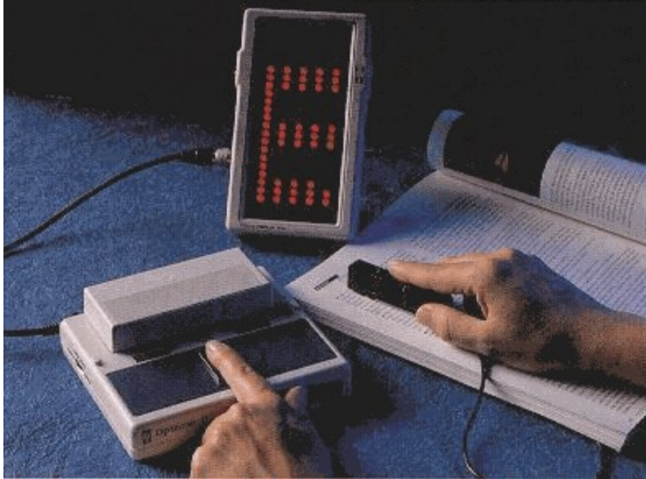
Figure 1-6: An image of Optacon device. This device was designed for reading letter-by-letter text. An Optacon has a camera which captures images of text/letter. Optacon has 24X6 vibrating pins and as a user moves the camera to scan a line, corresponding character are represented in Braille on the tactile array.
