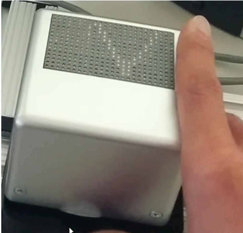
Figure 2-1: This figure depicts an image of the mini refreshable hyperBraille device. This device has piezoelectric vibrating pins which can go up/down at a very high refresh-rate. An image of some part of a triangle is being shown on the Braille device. This device also has the capability to perceive touch input from the user's fingertips.
