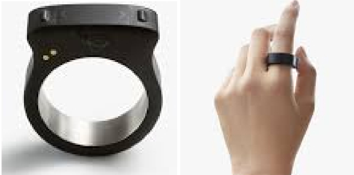
Figure 2-4: Snapshots of the Nod-ring. This Nod ring can be worn on fingers of a blind user and is very lightweight. This ring has motion sensors which can track its movement in XYZ directions. We have developed touch gestures such that vertical up movement of finger performs zoom-in of any tactile graphics on the Braille Device and vertical down movement of the Nod-ring performs zoom-out.
