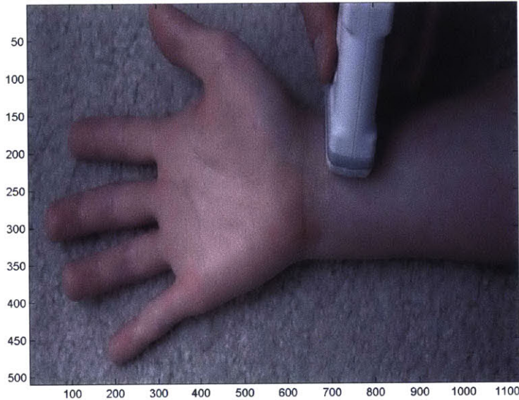
Figure 3-3: Experiment setup with a healthy female subject. The Doppler probe was placed on the radial artery in the wrist.
